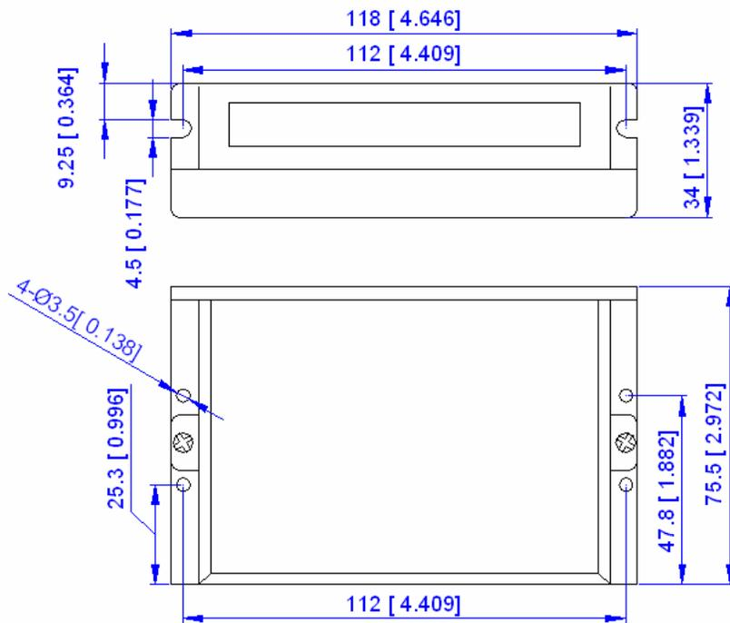
Figure 1: Mechanical specifications
