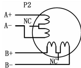
Figure 7: 6-lead motor full coil (higher torque) connections
