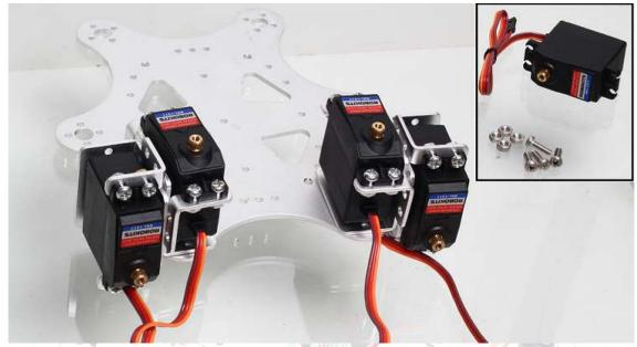
Step 6: Now again take the 2 x Servo Motors, 8 x M4 Screws and 8 x M4 Nuts and fix the Servo Motors on the two legs as shown in the below Image. Note the Orientation of the Servo Motors
