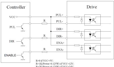
R=1K(Power>0.125W) if VCC=12V; R=2K(Power>0.125W) if VCC=24V; R must be connected to control signal terminal.
