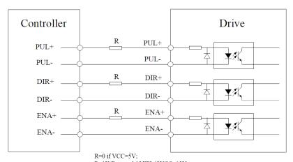
R=1K(Power>0.125W) if VCC=12V; R=2K(Power>0.125W) if VCC=24V; R must be connected to control signal terminal.
