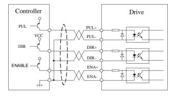
Figure 3: Connections to open-collector signal (common-anode)
