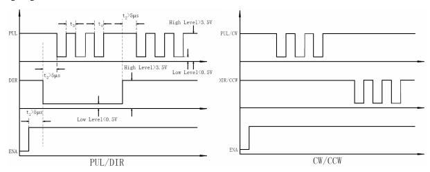
Figure 11: Sequence chart of control signals
