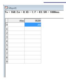
Dividing this value by 10 will give voltage in volts. In this case its 26.9V.
