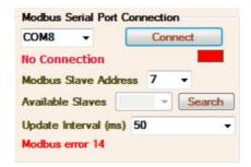
You may look in 'Devices and Printers' or 'Device Manager' for specific serial port of your device. The software supports serial ports up to COM32 only. If your device's port number is higher you can change it in - Device Manager > Ports (COM & LPT) > Double click on device name > Port Settings > Advanced > COM Port number
