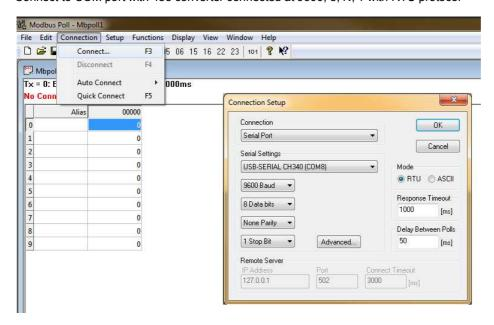
After connecting right click on cell and go to Read/write Definition...
