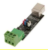
Modbus is connected with 9600bps baudrate, 8 bits, no parity and 1 stop byte (9600,8,N,1) in RTU protocol.
