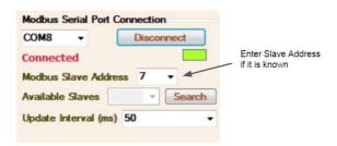
**2.** If slave address is not known or multiple drives with multiple addresses are connected on serial bus, click search button. This will search for all slave ids from 1 to 15. If any response is received from slave id it will give indication in status bar and list the drive in 'Available Slaves' drop down box.
